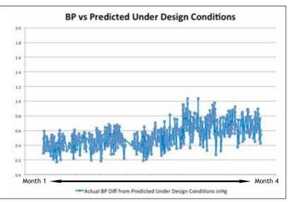
**Figure 5** - Condenser backpressure also dropped when the cooling tower fill was cleaned.
