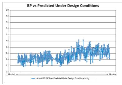
Figure 2 - Condenser Backpressure increased.
