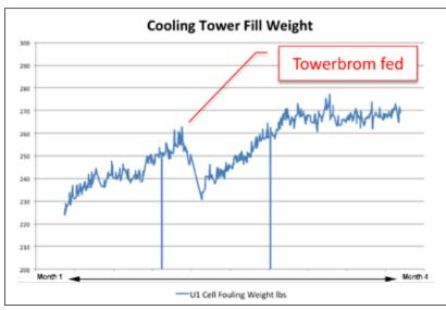
**Figure 4** - The actual cause of the problem was microbial fouling in the cooling tower. When the deposits were removed, the weight of the cooling tower fill dropped. When the biodispersant program was discontinued, the weight increased again.
